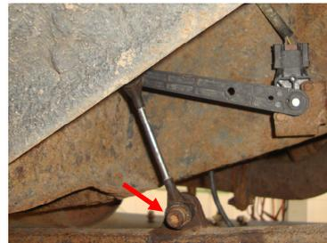
**7.** At each side of the vehicle, fit a height sensor bracket to the outside of the flange on the vehicle radius arm, using a new M8 x 30 flange bolt and nyloc nut...
