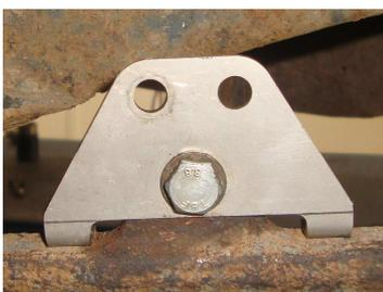
**8.** At each side of the vehicle, **LOOSELY** attach the height sensor connecting rod to the bracket using a M8 x 40 flange bolt and nyloc nut - choose the bracket hole nearest to the front of the vehicle...
